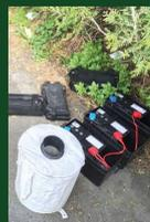
BG-Sentinel trap (Biogents) with batteries © ITG
